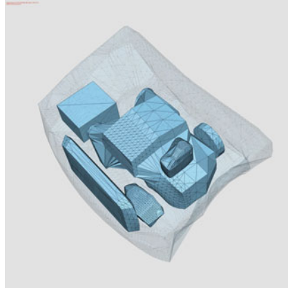
Fig. 3.8 Vehicle layout for the battery cells arranged to nine columns and eight rows, and the maximum importance given to the vehicle level [12]
