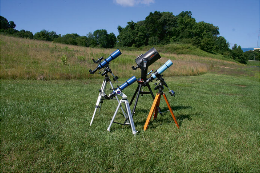
Fig. 2.16 The author's telescopes featuring an Alt-Az with slow motion controls, two German equatorials, and computerized GOTO mount (Adam Chen)
