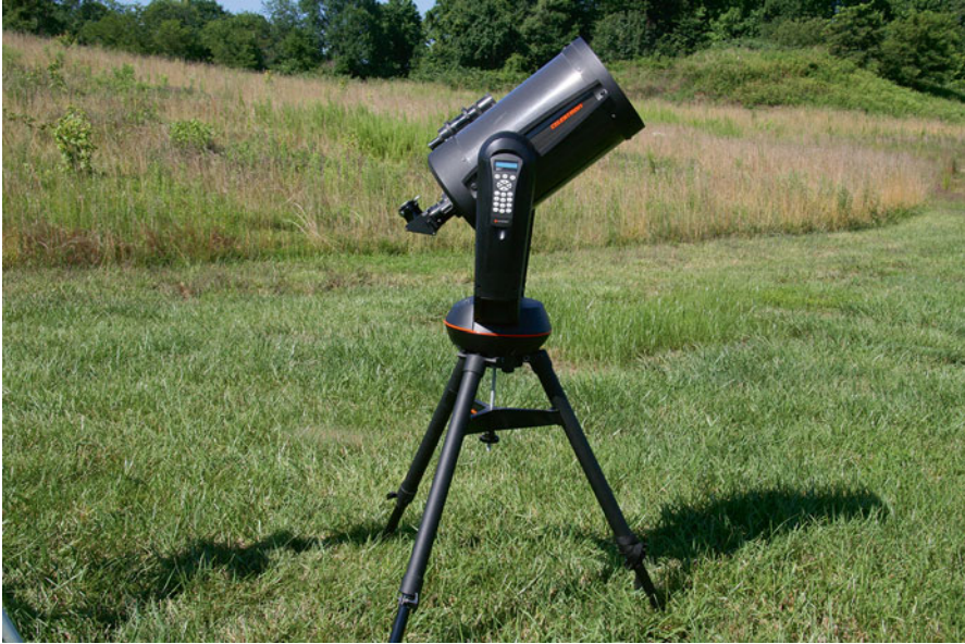
Fig. 2.20 Computer GoTo mounted Schmidt-Cassegrain (James Chen)
