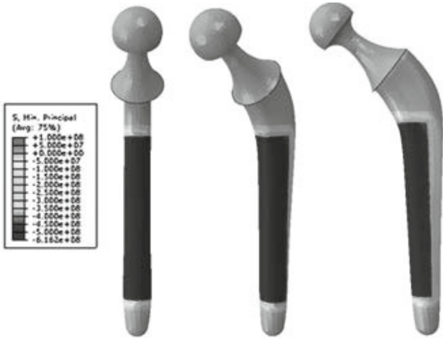
Fig. 3. Treatment geometry and colour scale presentation of the minimum principal superficial residual stresses induced in the considered hip replacement by LSP
