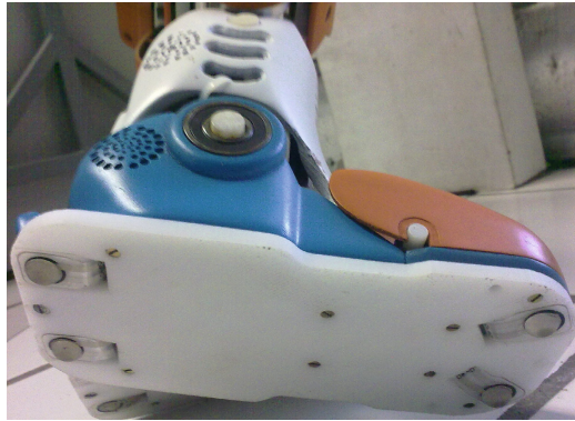
Fig. 5. Four force sensors are located under each foot
