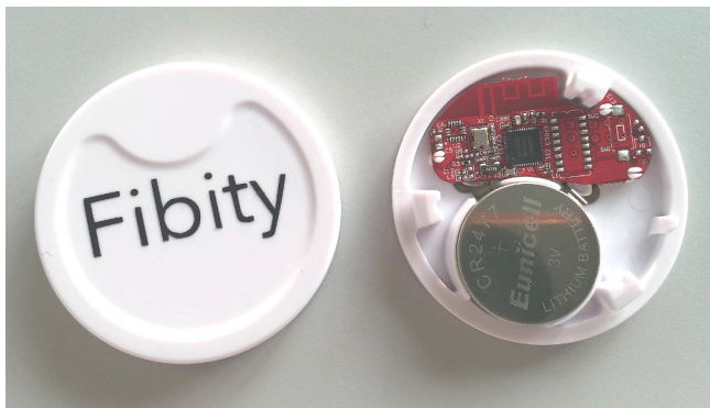
Fig. 1. BLE beacon. The simple circuitry is visible. It is powered by a usual 3 volts clock battery. The beacon diameter is about 5 cm.
