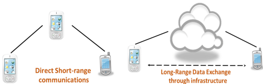
Fig. 2. Two approaches proposed for use case implementation for the Portuguese partners use-case, when short-range is possible (left) and when long-range/infrastructure only is possible
