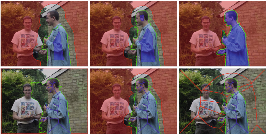
Fig. 4. Segmentation examples using WSVol for the 6 marker combinations. In each figure the background and foreground marker are respectively depicted in red and blue while the contour of the segmentation result is in green.
