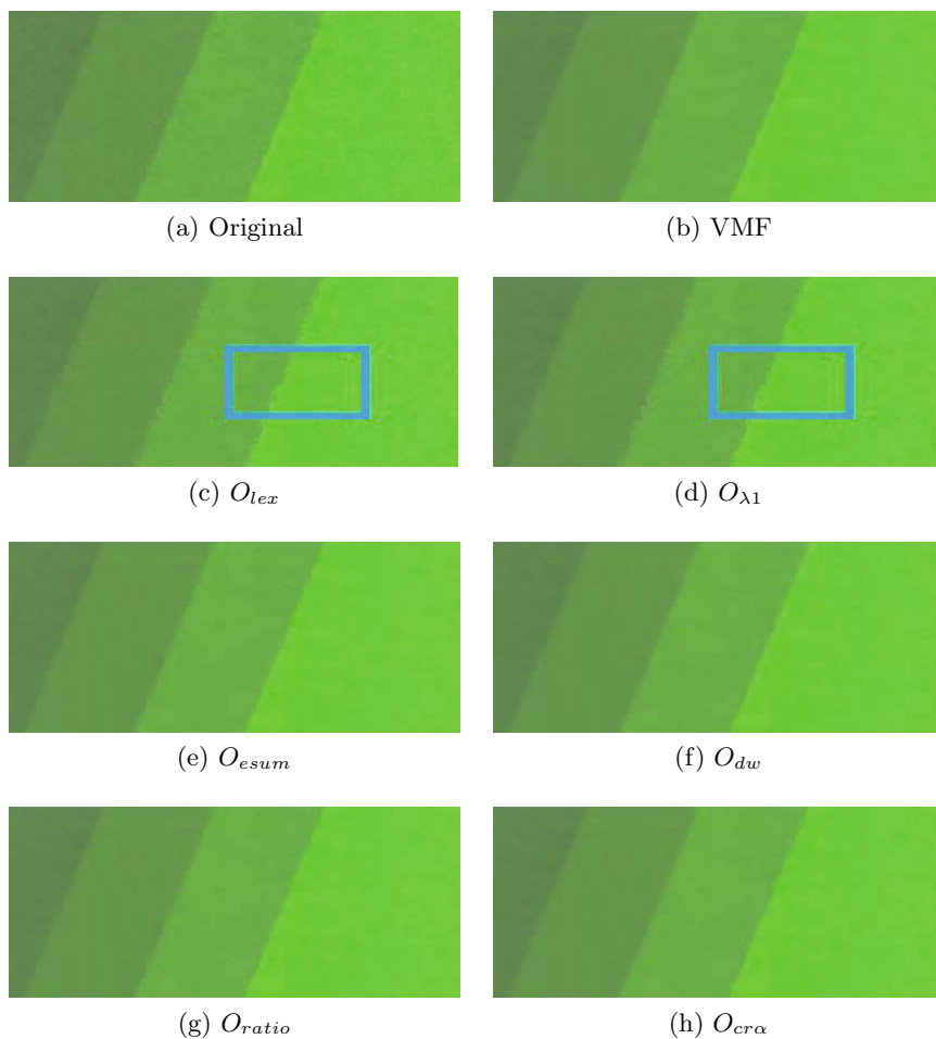
Fig. 4. Results of applying VMF and several spectral median filters with different ordering relations on pigment P3. Similar to the case of P2 in Fig. 3, the spectral median filters that are based on ordering relations O_{lex} and O_{\lambda_1} are also not able to maintain the edges that exist between two color shades, see regions inside the blue squares.
