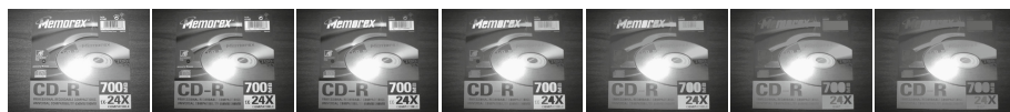
Fig. 4. Some images of a scale-space generated with markers produced by alternate sequential filtering
