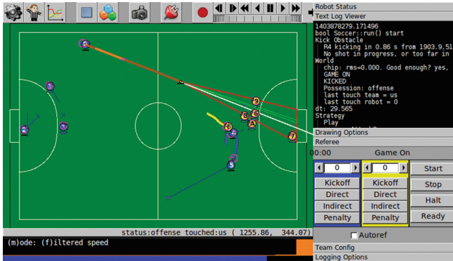
Fig. 2. A snapshot of our sophisticated graphical visualization program used for simulation, monitoring the real robots, and replaying logged game data.
