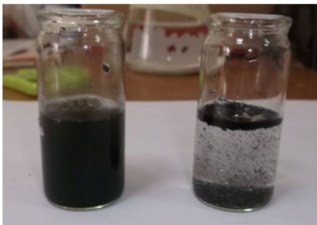
Fig. 33.6 Graphene oxide with hydrazine ( left ) and reduced graphene oxide ( right )
