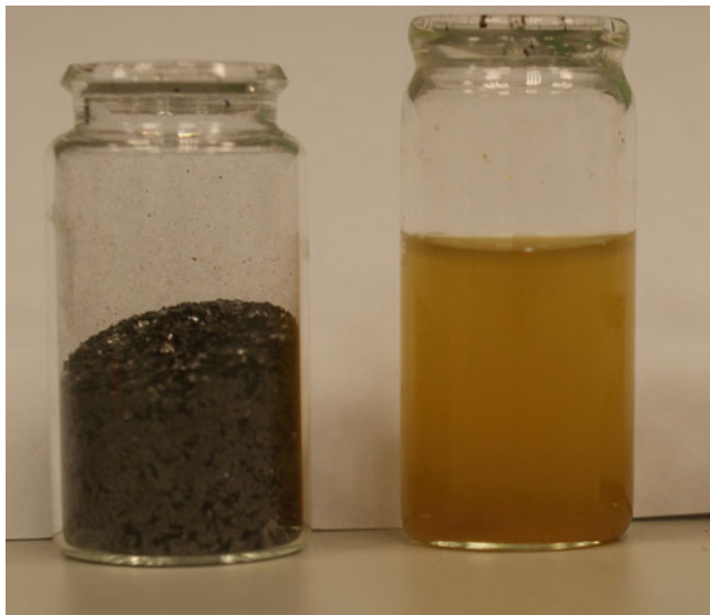
Fig. 33.5 Graphite powder ( left ) and graphene oxide suspension ( right )
