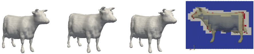
(a) Least-squares (b) Our model (c) p-ref, ours (d) Hierarchy Fig. 3. Refinement: 3(a) h-refinement of least-squares model 2(c); 3(b) h-refinement of our model 2(d); 3(c) p-refinement of 3(b). The Hierarchical mesh 3(d) with first-level elements in blue, second level in gray, and third level in red.
