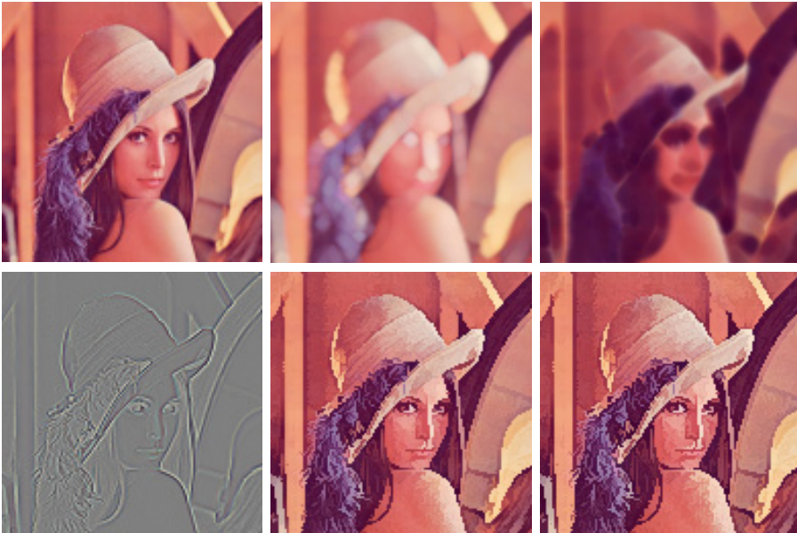
Fig. 3. Top row. Original Lena image, and results of dilation and erosion computed with the RT scheme. Bottom row. Morphological Laplacian and results of five and ten iterations of shock filtering with the RT scheme.
