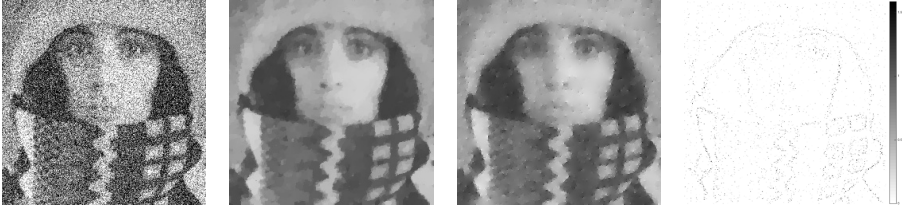
Fig. 5. Noisy image (Gaussian noise, variance 0.05, left), ROF denoising result ( \lambda = 5 , middle left), SVF denoising result ( \lambda = 4 , middle right), norm of vector field v in SVF model (right).
