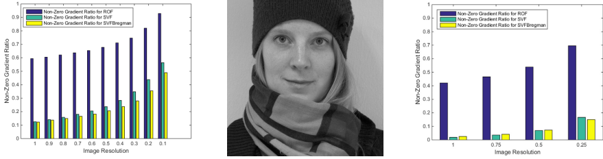
Fig. 3. Comparison of the Non-Zero Gradient Ratios of the SVF ( \lambda = 10 ), the SVF-Bregman ( \lambda = 1 and 5 Bregman Iterations) and the ROF ( \lambda = 10 ) algorithms for the Trui test image (left) and an additional test image of size 1024x1024 pixels (right). The latter test image is displayed in the middle.
