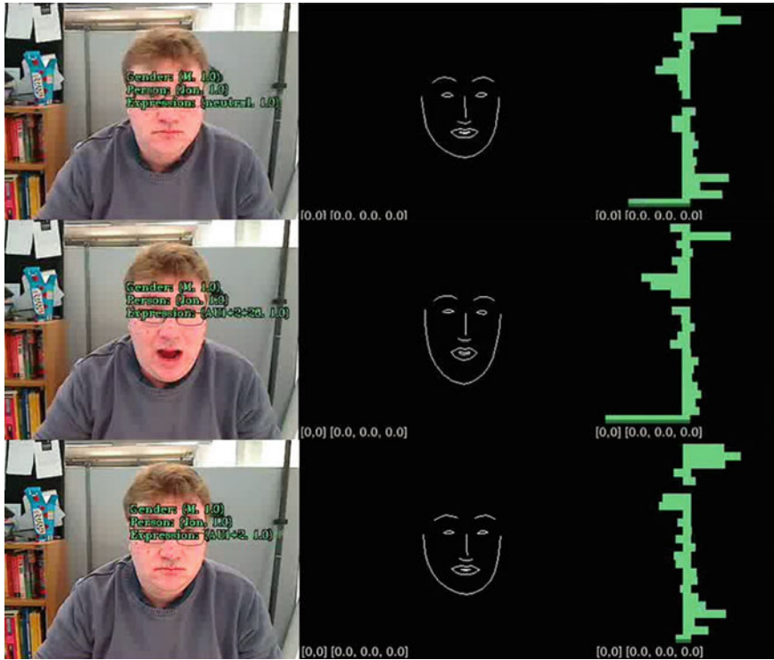
Fig. 2 Recognition of expressions in a laboratory setting using a CLM. The bars on the right illustrate the values of the parameter vector which define the shape of the model shown in the centre . Automated fitting techniques are used to adjust the values in the parameter vector so that the generated shape optimally matches the face in the image on the left
