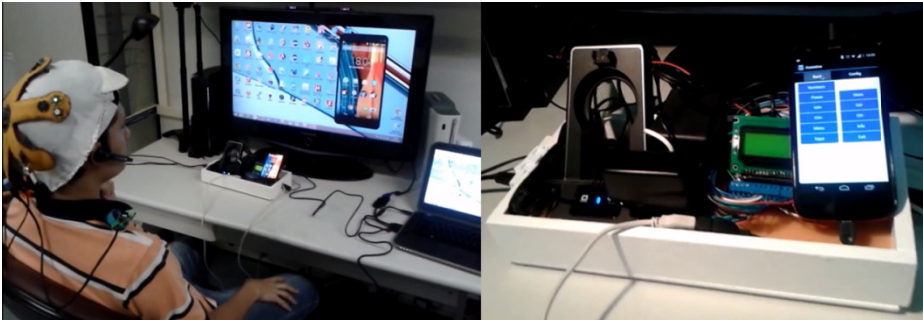
Fig. 2. Our AT prototype platform: on the left, a user wearing the cap to control a lamp, a TV and a computer; on the right, the dock station connected to a mobile phone with our app.
