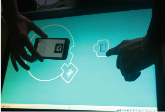
Fig. 1. An example of a workflow that can be assembled using our prototype; widgets are displayed on the smartphone once a new piece requiring some user input is assembled
