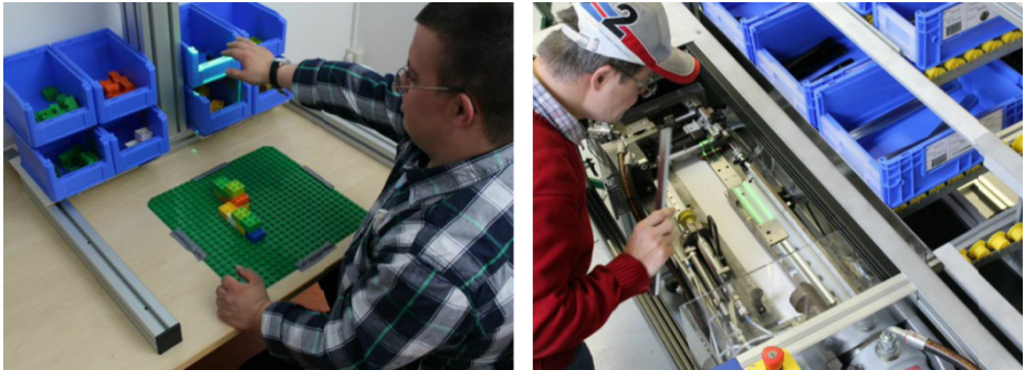
Fig. 1. The figure shows the MotionEAP system that allows semantically rich programming by demonstration. The system observes actions and can replay recorded sequences adapted to a new environment and users with varying performance. Left: test scenario in the lab; right: application in an industrial production process (photos courtesy to Markus Funk).
