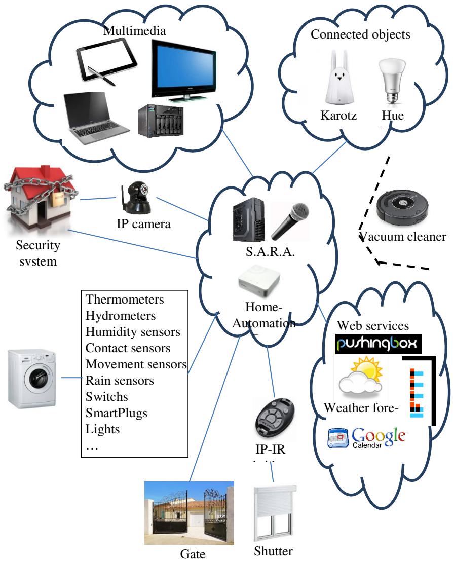
Fig. 1. Devices, services and their connections
