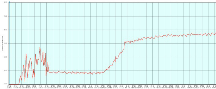
Fig. 7. Example of the power P [kW] curve of the grinder after design and process-related modifications and achievement of stable working process
