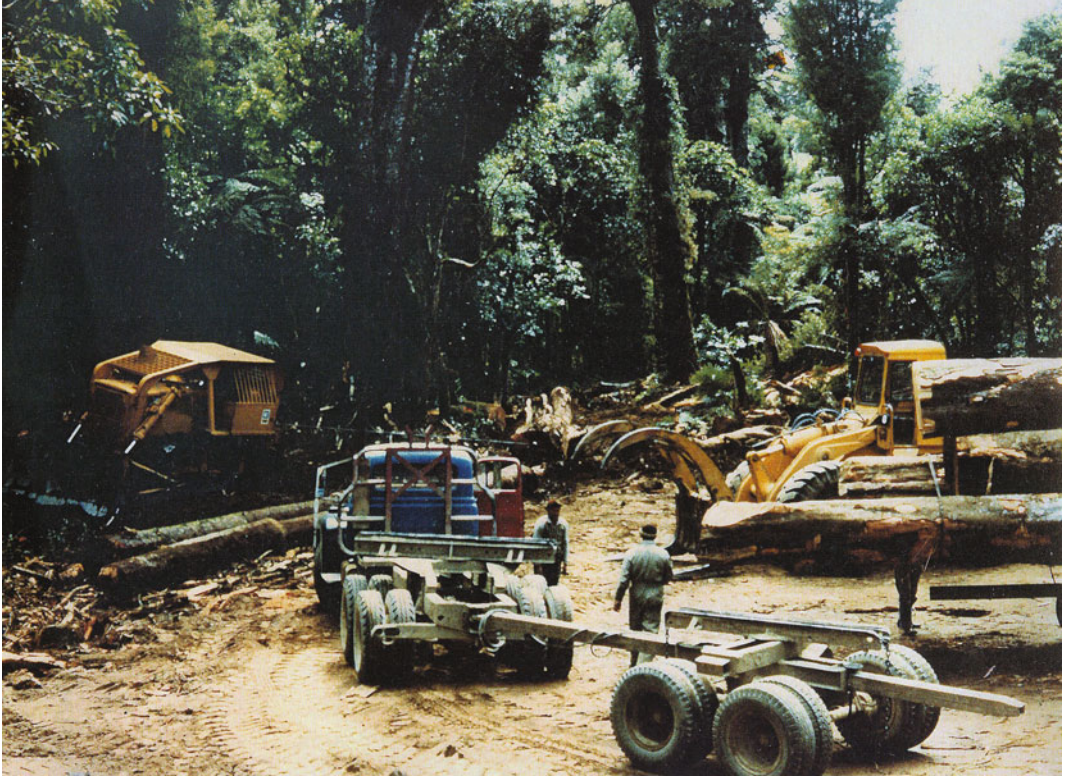
Fig. 7.16 By 1977, logging operations at Pureora were fully mechanised. A D7 tractor has brought rimu logs to a collection area, where a loader stands ready to lift the logs directly on to a waiting truck. The wasteful and dangerous
