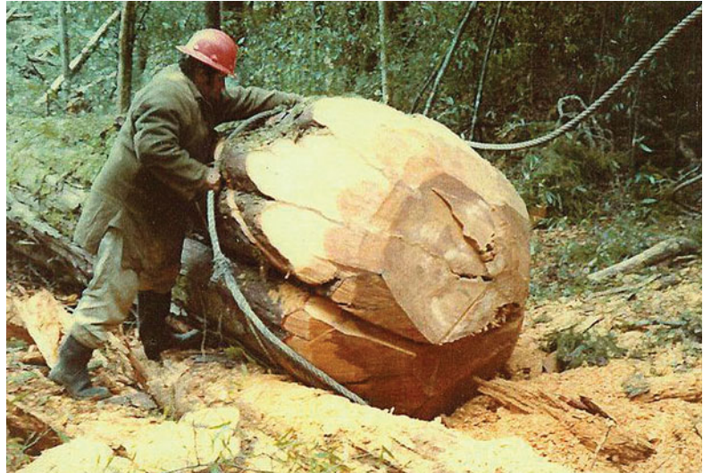
Fig. 7.11 A log being prepared for hauling. The leading end has been sniped (rounded), and a “D” groove cut to secure the steel cable with which the hauler will pull the log from stump to skid. Crown Copyright, Department of Conservation Te Papa Atawhai. Photographer unknown
