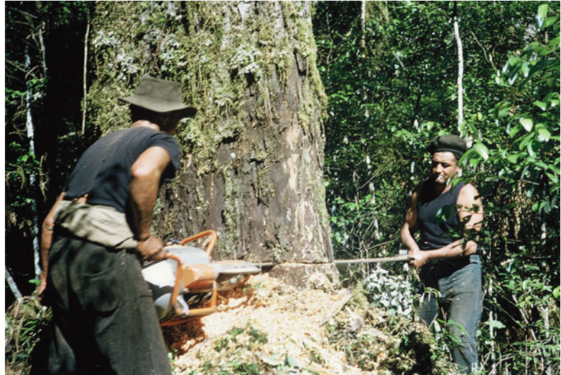
Fig. 7.9 Using an early two-man Mercury chainsaw to fell a rimu. Safety helmets were being introduced, but were unpopular with the bushmen. Photographer unknown, copyright assumed SCION image 8043889
