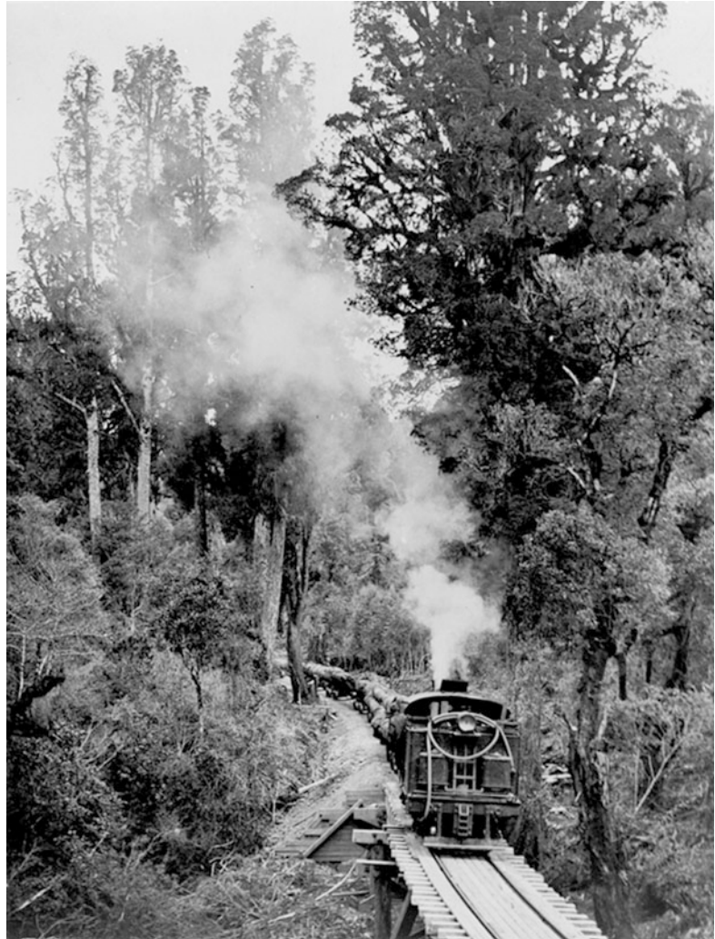
Fig. 5.11 E&B's Climax 1650 bush lokey working on the Ongarue tramway in 1929, surrounded by tall forest. Hamilton City Library, image 1613
