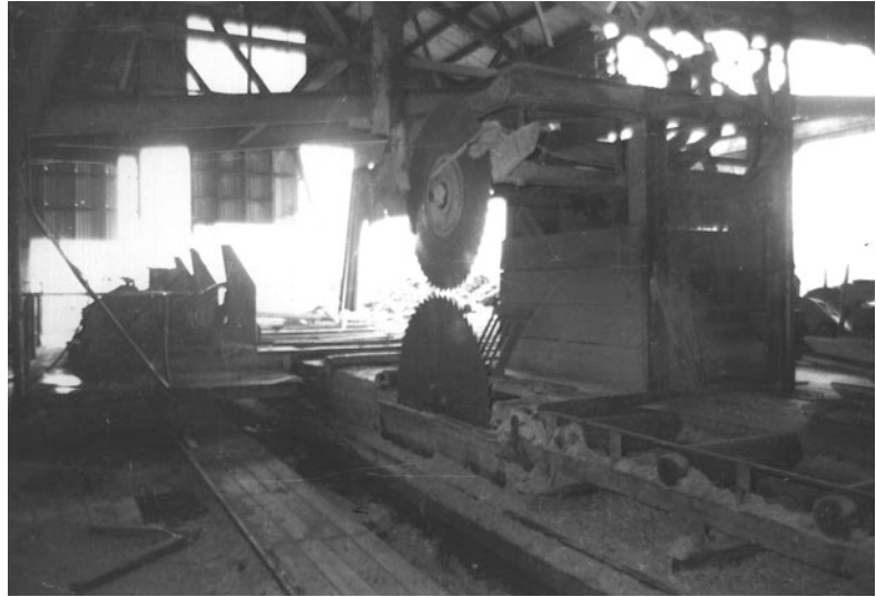
Fig. 7.17 A breakdown bench with a headrig equipped with twin circular saws, used by Odlin's mill at Pureora (built in 1947) and also by many other older mills. Crown Copyright, Department of Conservation Te Papa Atawhai. Photographer unknown
