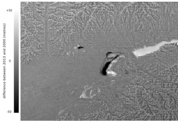
Fig. 4 Difference between DEM from Pleiades (from year 2013) and SRTM (from year 2000) over Angren, Uzbekistan—difference in landslide areas goes up to 50 m affecting InSAR detection ability (Lazecký et al. 2013)
