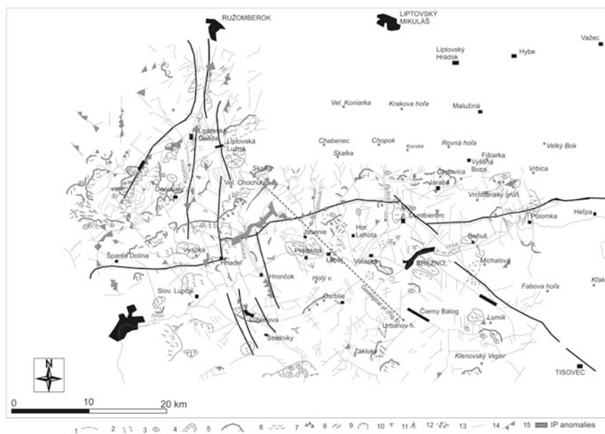
Fig. 4 Analysis of geodynamical phenomena. Legend 1 slope deformations general, 2 talus creep, 3 block rifts, block fields, 4 individualized blocks, 5 scarps, 6 landslides, 7 alluvial fan, 8 gully erosion, 9 erosion edge, 10 sheet erosion, 11 proluvial cones, 12 sinkholes, karst valleys, 13 linear boundaries (after remote sensing), 14 facets, 15 zone with height IP (induced polarization) anomalies
