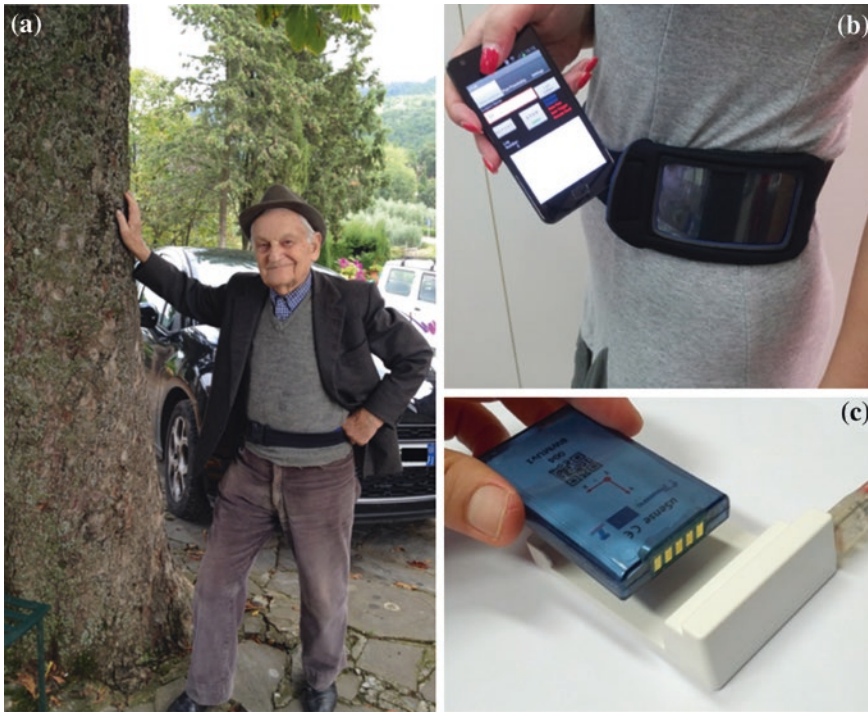
Fig. 1 a Elderly person wearing the smartphone as a monitoring unit by means of a custom elastic waist belt. b Waist belt used for wearing the smartphone for both activity monitoring and functional assessment. c FARSEEING wearable monitoring unit specifically designed for long-term monitoring of people at high risk of falling
