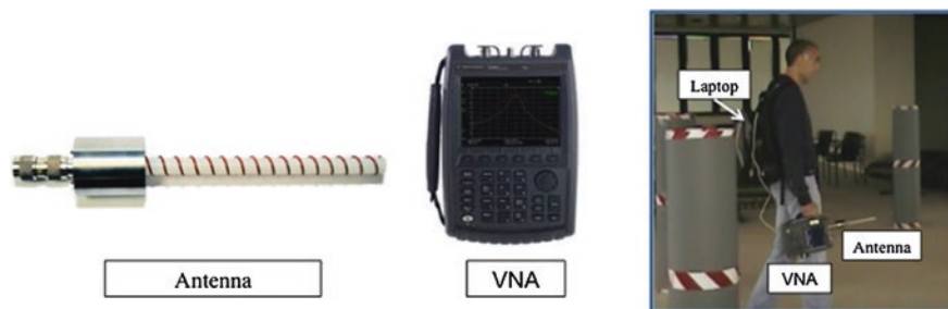
Fig. 4 Photos of the EM obstacle detection sensor. The homemade antenna and the VNA ( left ) the system in use ( right )
