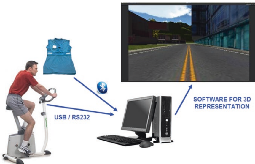
Fig. 2 Overall architecture for fatigue level control at constant Heart-Rate
