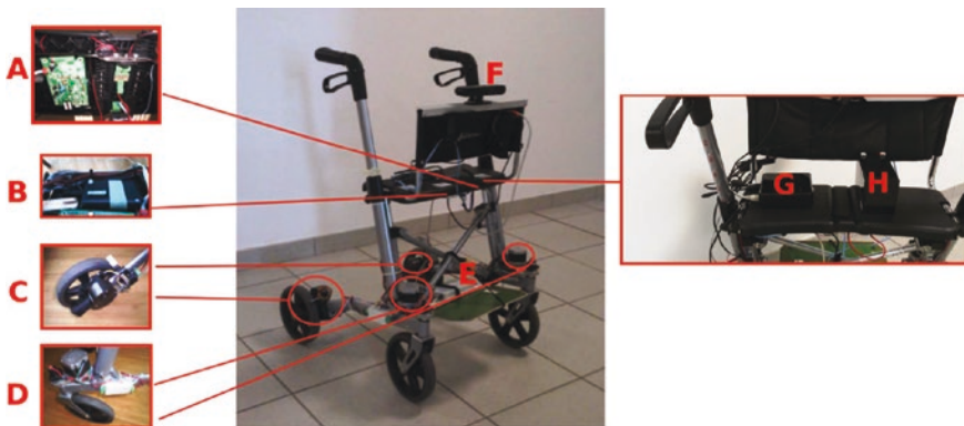
Fig. 1 The c-Walker prototype along with its main components, i.e. Beaglebone platform (A), IMU (B), encoders (C), motors (D), RFID Reader (E), Camera (e.g. Kinect) (F), Barebone platform (G), and main battery (H)
