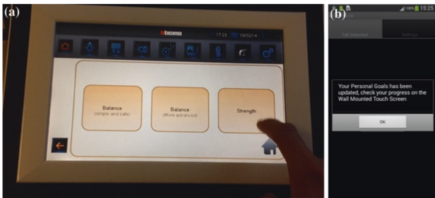
Fig. 2 a Wall-mounted touchscreen used for providing tips, feedbacks, and exercise guidance to the user. b The Smartphone provides reminders and inform the user about the content available on the wall-mounted touchscreen
