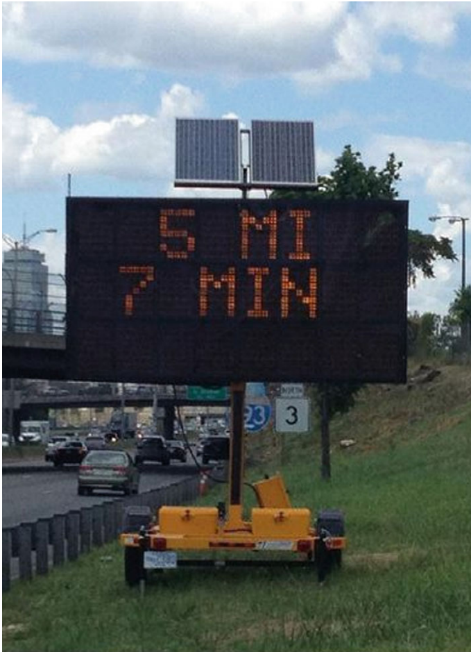
Fig. 1 A portable variable message sign displaying travel times on Interstate 93
