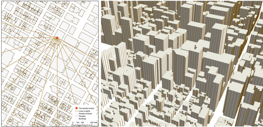
Fig. 4 Point matrices on the façades and the lines of sight from a sample point
