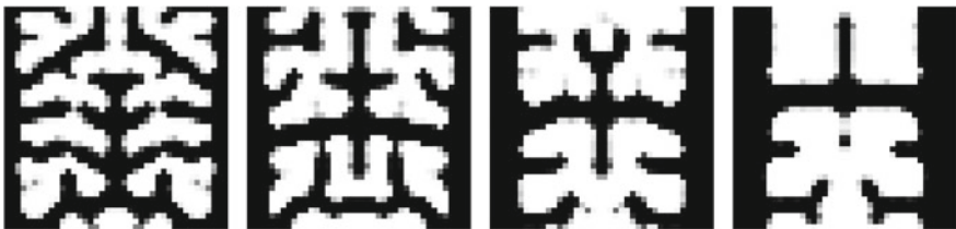
Fig. 5 Optimized heat sink coarse cell topology for 4 \times 4 , 8 \times 8 , 16 \times 16 and 32 \times 32 coarse cells
