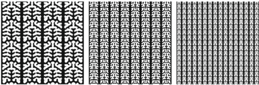
Fig. 4 Optimized heat sink topology for 4 \times 4 , 8 \times 8 , 16 \times 16 coarse cells
