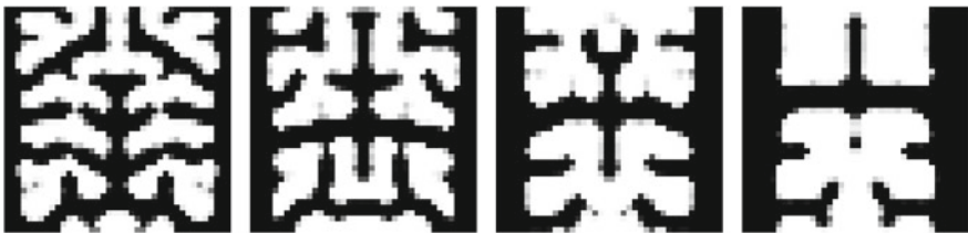
Fig. 5 Optimized heat sink coarse cell topology for 4 \times 4 , 8 \times 8 , 16 \times 16 and 32 \times 32 coarse cells
