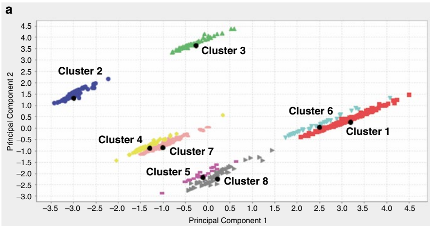
Fig. 14.1 The training data projected onto two-dimensional planes formed by two of its first three principal components: (a) principal components 1 and 2; (b) principal components 1 and 3; (c) principal components 2 and 3 (From Azmandian et al. [22])
