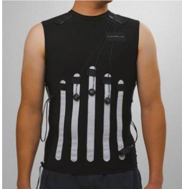
Fig. 11.13 An array of optically-tracked LED markers to measure breathing
