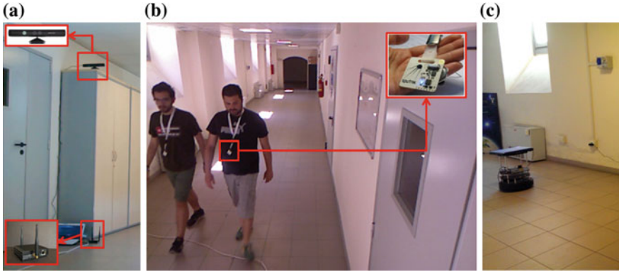
Fig. 10 Real experiment: a fixed node composed by a Kinect and a RFID receiver, b two RFID tags, c a Turtlebot robot equipped with a laser range finder
