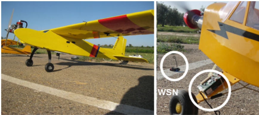
Fig. 11 Left Megastar fixed-wing UAV used in the experiments. Right Piper fixed-wing UAV used in experiments. Detail of the on-board and deployed WSN
