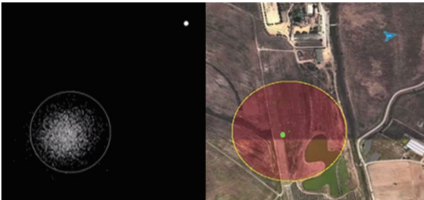
Fig. 6 Ground visualization tool. Particle distribution and UAV position ( left ); map visualization ( right )
