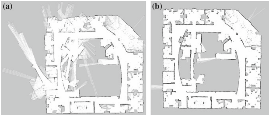
Fig. 6 Mean error in the Intel Research Lab dataset with N = 90 . a Classical approach. \bar{\epsilon}_{trans} = 0.065 \pm 0.38 (m), \bar{\epsilon}_{rot} = 2.809 \pm 6.539 (deg), b Stateful MT approach with K = 2 . \bar{\epsilon}_{trans} = 0.028 \pm 0.037 (m), \bar{\epsilon}_{rot} = 1.977 \pm 1.817 (deg)
