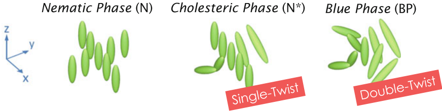
Fig. 9.2 Schematic depictions of director distribution in nematic phase (N), cholesteric phase (N*) and blue phase (BP)
