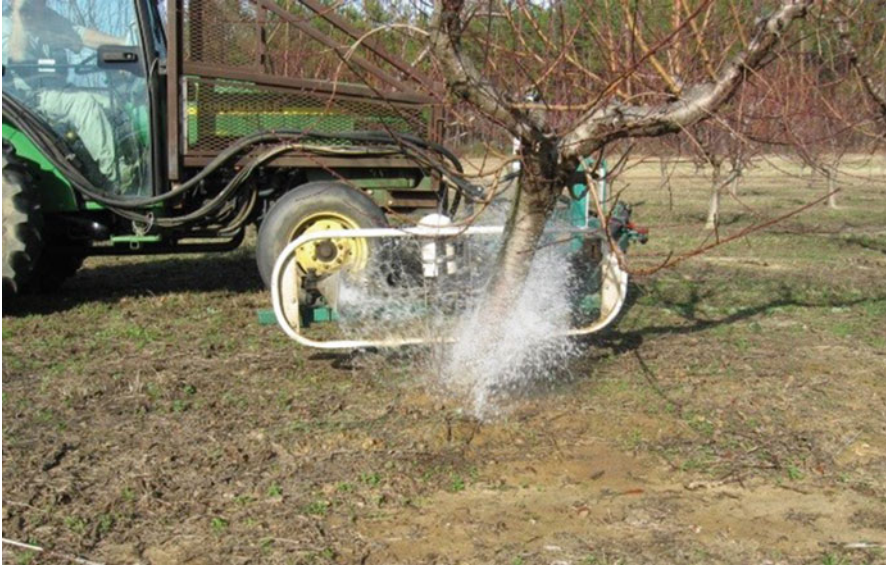
Fig. 9.1 Trunk sprayer applying nematodes to the base of a peach tree in Georgia (Photo credit: Ted Cottrell, USDA-ARS)
