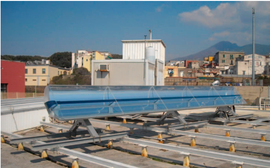
Fig. 30.1 The Absolicon X10 PVT collector operating at the ENEA Portici Research Centre
