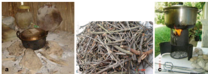
Fig. 82.7 a 3-stone fireplace. b Renewable harvested firewood for cooking with the green stove. c: The green stove is used to boil 5 L of water [5]. Portability and self-regulating air supply are the advantages
