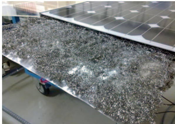
Fig. 56.3 PV/T collector with stainless steel wool heat exchanger
