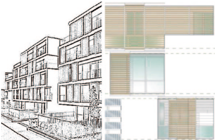
Fig. 83.7 Moveable shading device along the whole facade and different seasonal way to use them
