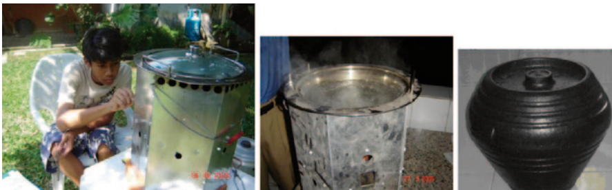
Fig. 82.5 Save80 stove, boiling water inside the stove and the wonder box
