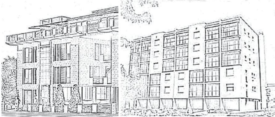
Fig. 83.6 Sketches with different configuration of the greenhouse: glazing and shading device for each loggia of the building
