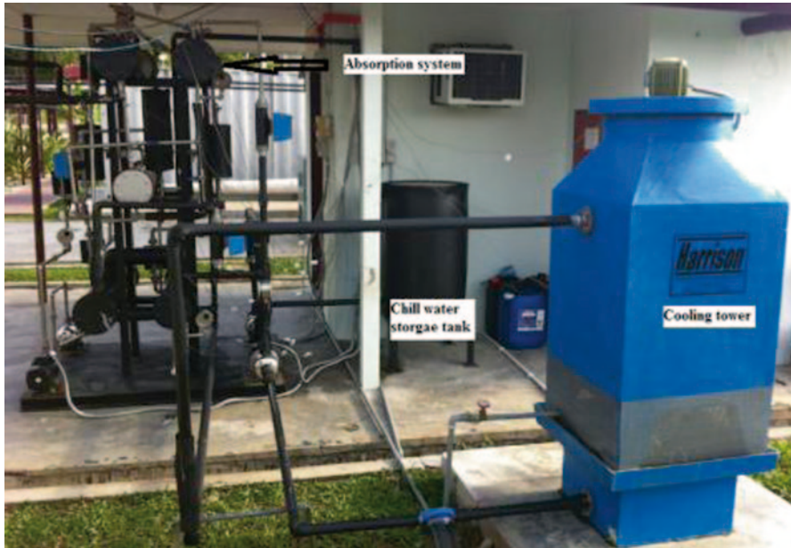
Fig. 54.2 Modified combined ejector–absorption cooling system
