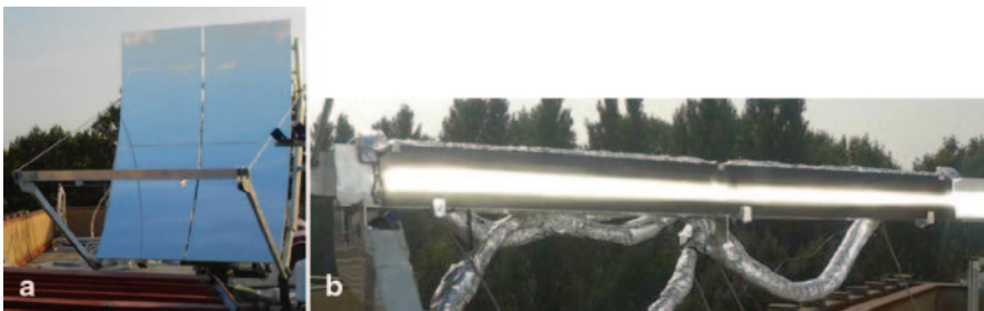
Fig. 63.3 a Prototype of the PTC collector. b The thermal receiver
