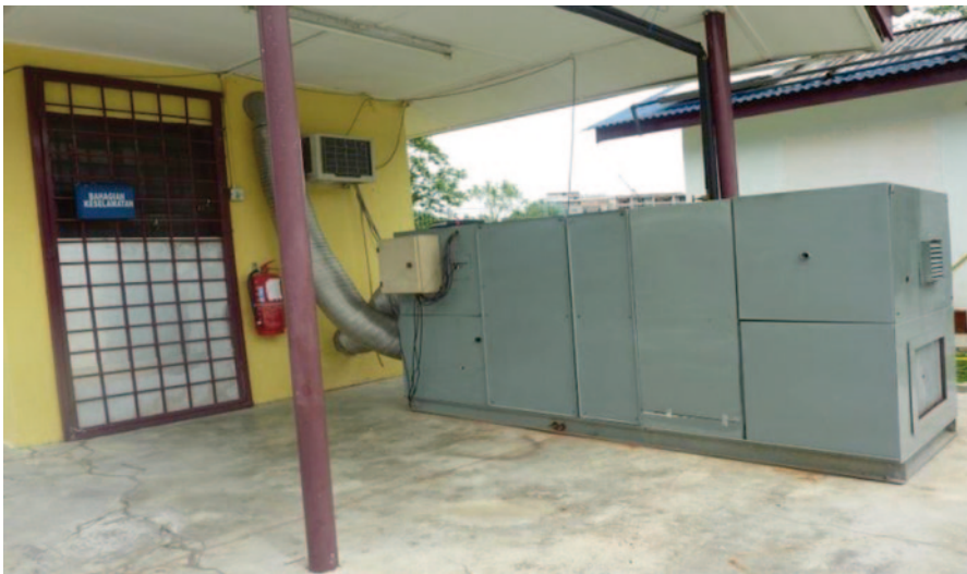
Fig. 68.1 Experimental setup of one-stage desiccant cooling system in technology park of UKM
