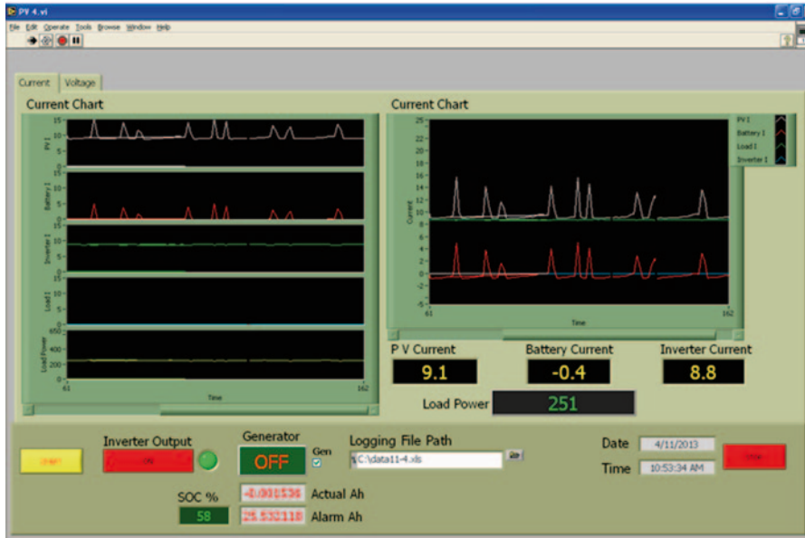
Fig. 37.7 Program screen showing load supported by PV and batteries
