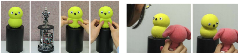
Fig. 7 Keepon, a simple robot with a soft body to engage in non-verbal social interaction [17]
