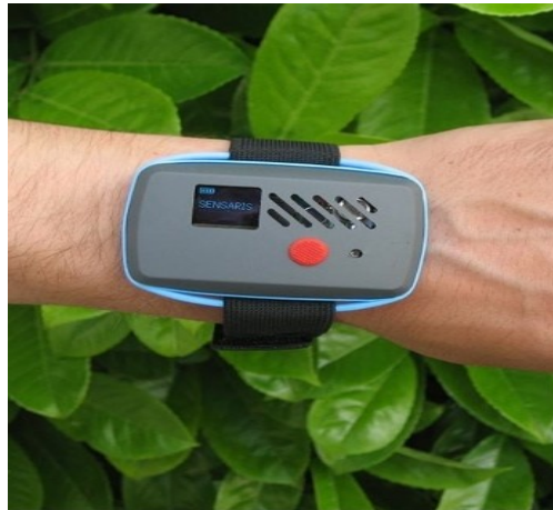
Fig. 9 Wrist worn sensor used for hand motion detection [95]
