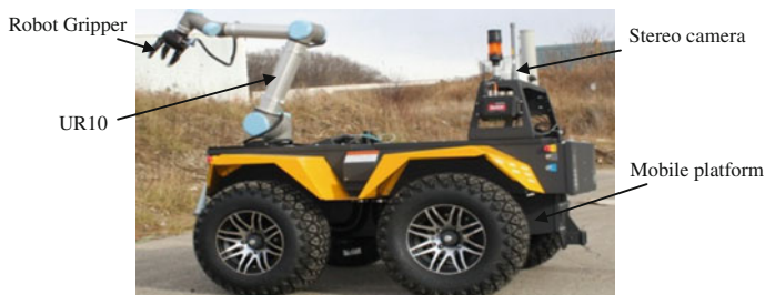
Fig. 2 A mobile manipulator system Grizzly ® for automated twistlock handling [9]
