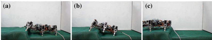
Fig. 6 Snapshots of the hexapod prototype with climbing behavior: a Start climbing. b Front legs on the stair. c Climb entirely onto the stair
