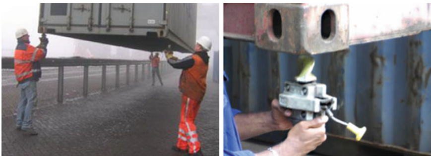
Fig. 1 Examples of dockworkers manual deconing twistlocks on container corner castings
