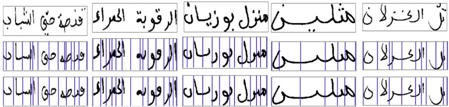
Fig. 18. Samples of word images after the over segmentation stage and after the neural validation
