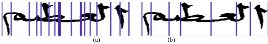
Fig. 5. a) Initial prospective points, b) Segmentation points after applying the ACW and open hole rules
