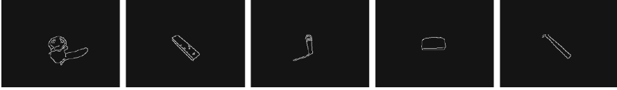
Fig. 4. The above figure shows the images after setting rectangular masks on the Canny Edge Detector processed gray images (Color figure online)
