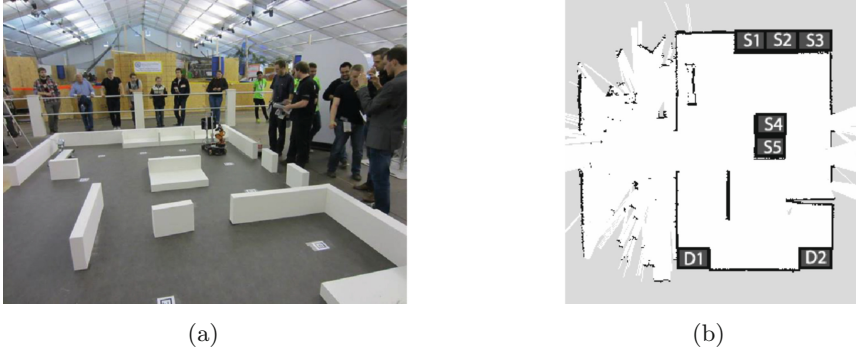
Fig. 1. (a) RoboCup@Work arena with extra static obstacles. (b) Map of the arena. Annotated with service areas.
