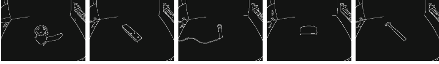
Fig. 3. The above figure shows the images after being processed by the Canny Edge Detector
