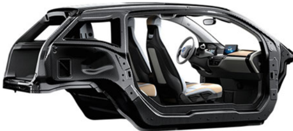
Fig. 2 Lightweight passenger cell of BMW I3 made of carbon (Source BMW website)
