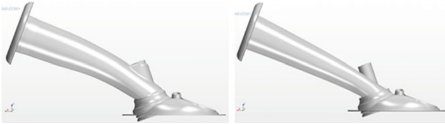
Fig. 3 Intake port design for the Fill port ( left ) and the Tumble port ( right )
