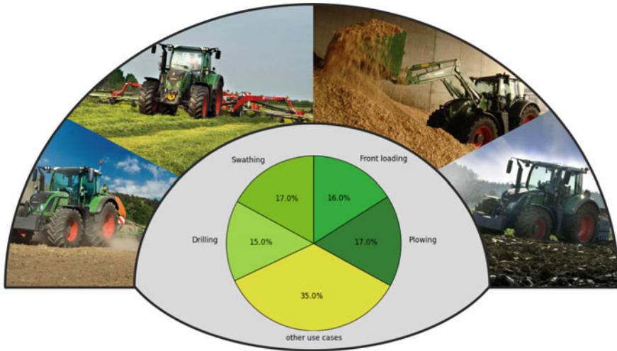
Fig. 2 Distribution of duty cycle time shares in an application area ( Sources Scherer, AGCO Fendt)
