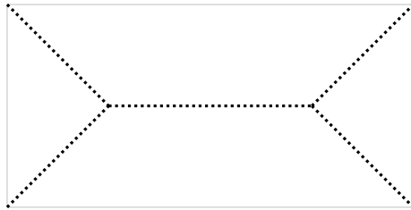
Fig. 7. Medial Axis Transform of the gray rectangle consists of five line segments shown on the picture
