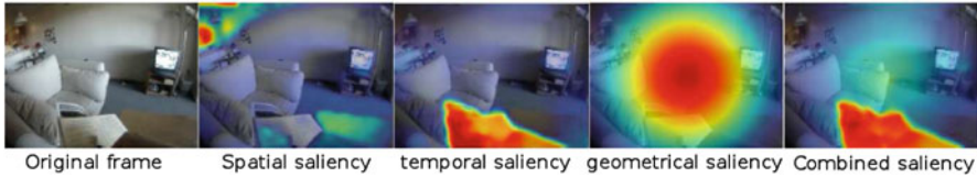
Fig. 3 Illustration of the different saliency cues (geometrical, spatial and temporal) composing the spatio-temporal saliency maps from [5]
