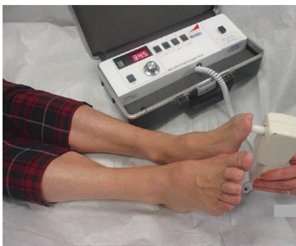
Fig. 1.9 Neurothesiometer which delivers a vibratory stimulus that increases as the voltage is raised until the patient notes the vibration sensation and this is deemed the vibration perception threshold
