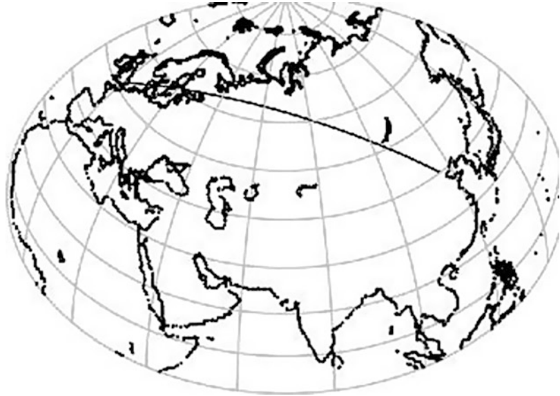
Mathematical Foundations of GIS, Fig. 3 Great circle route from London to Beijing
