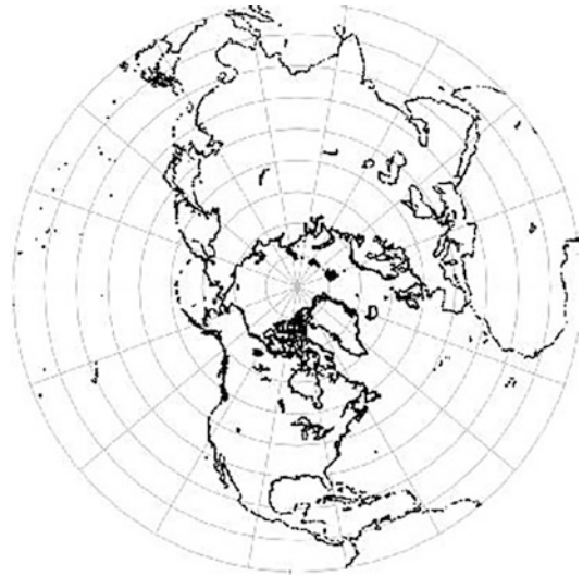
Mathematical Foundations of GIS, Fig. 8 Azimuthal equidistant projection of the northern hemisphere
