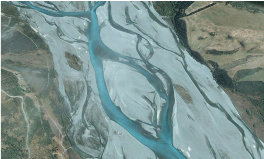
Fig. 15.4 Bifurcations and confluences in the Rakaia River (New Zealand); braidplain width is about 900 m (from Google Earth)
