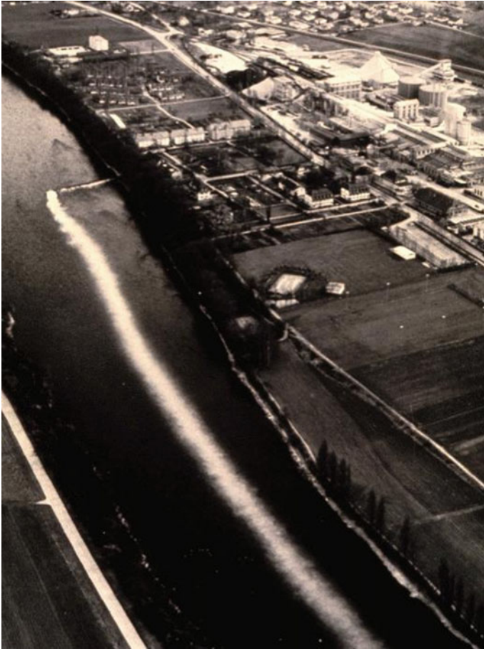
Fig. 24.3 Aerial photograph (ca. 1960) of an industrial discharge located near the middle of the regulated River Rhine upstream of Lake Constance (Bodensee); photograph courtesy of D. Vischer, Zurich; source Jirka and Weitbrecht (2005)
