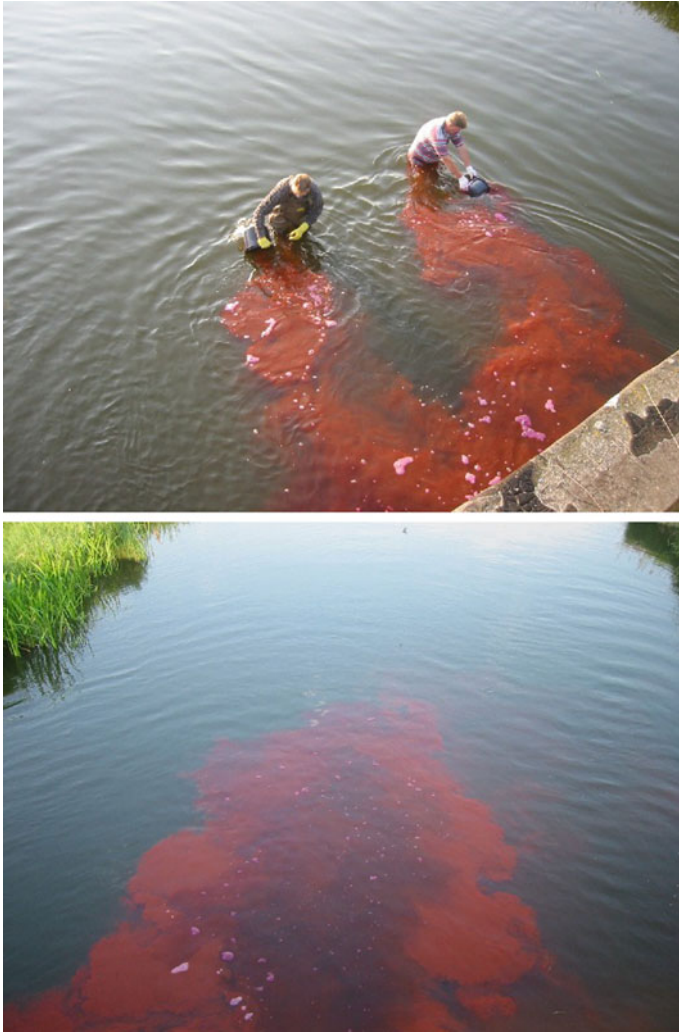
Fig. 24.2 Tracer test performed in a natural Narew river in north-east Poland in June 2005 (Rowiński et al. 2007, 2008); dye release ( top figure ), section directly behind the discharge ( bottom figure )
