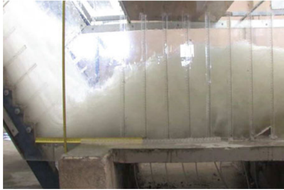
Fig. 9.2 Model investigation on stilling basin performance downstream of a steep stepped spillway (Bung et al. 2012), channel width is 1 m to avoid model effects
