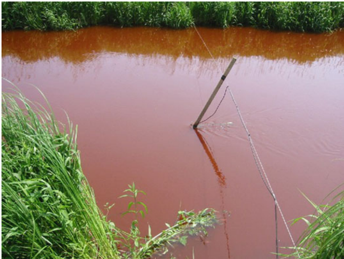
Fig. 24.5 Tracer test performed in a natural Narew river in north-east Poland in June 2005 (Rowiński et al. 2007, 2008); after complete mixing along the river width
