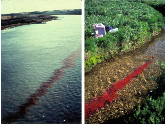
Fig. 24.4 Tracer study of horizontal mixing in Missouri river in USA, source Holley (2001) ( left figure ); Rhodamine dye study of hydrology of stream-lake interactions (Spring Creek lake), source http://www.aslo.org/ , author: Prof. Wayne Wurtsbaugh ( right figure )
