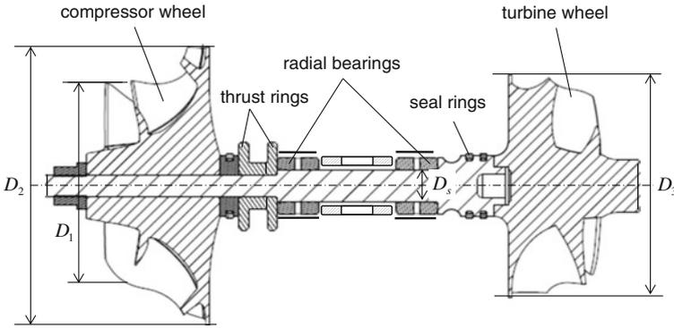
Fig. 10.2 Setup of the CHRA of a turbocharger
