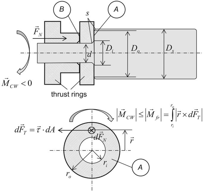
Fig. 10.3 Friction torque versus compressor wheel torque
