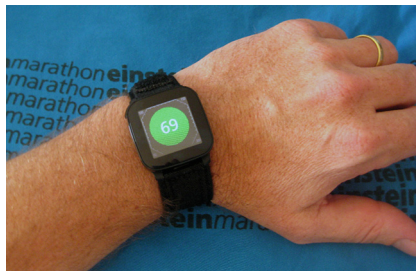
Fig. 11. Remote wrist display for Android smartphone. This device can perfectly complement the heart rate monitoring UI for endurance sports like, e.g., distance running or skating.
