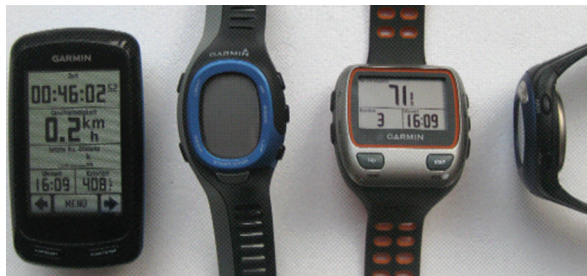
Fig. 2. Typical sports computers and watches, which can perform heart rate monitoring as main feature or in addition to other functionalities.
