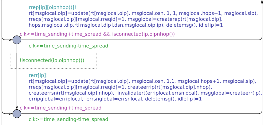
Fig. 3. Extract from Handle(ip, art[ip]) model for AODV at RREQ message
