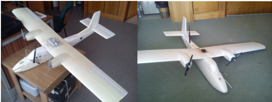
Fig. 7 Two fixed-wing UAVs which were used in the experiment. Antennas of 868 MHz radio modems are visible at the nose and the tail. The rudder of the UAV on the left picture has a built-in antenna for 2.4 GHz modem. In the second UAV 2.4GHz antenna is under the left wing
