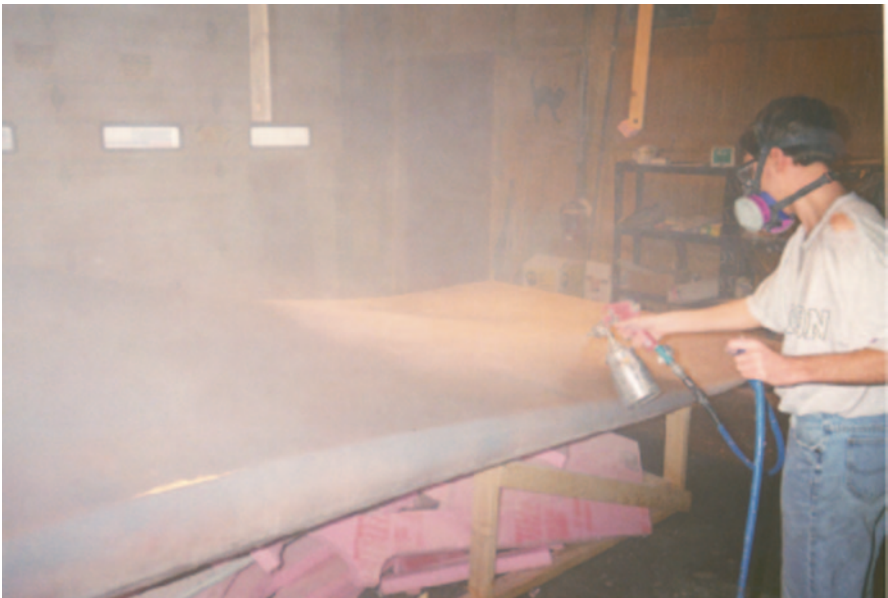
Fig. 11.12 Spraying primer. (Brian Lisiecki)
