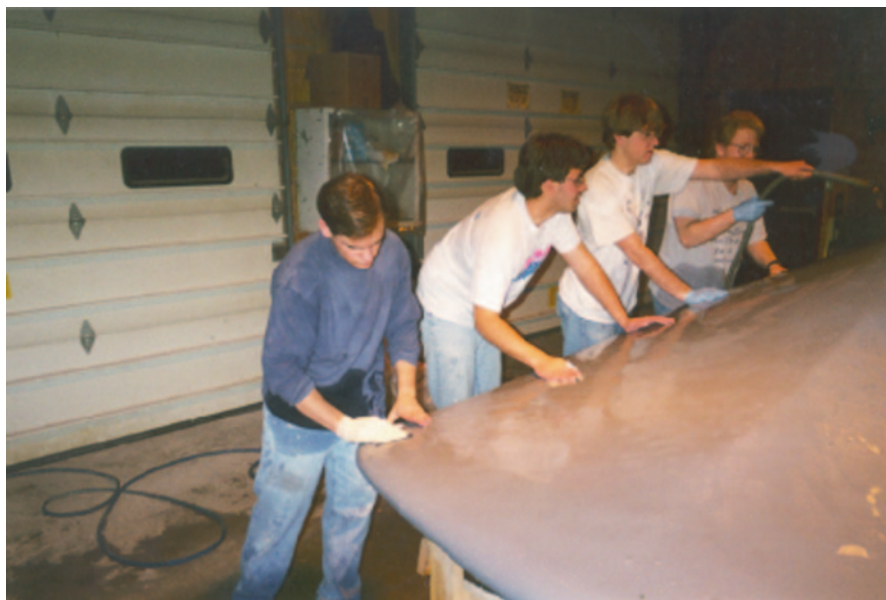
Fig. 11.13 Wet-sanding plug. (Brian Lisiecki)
