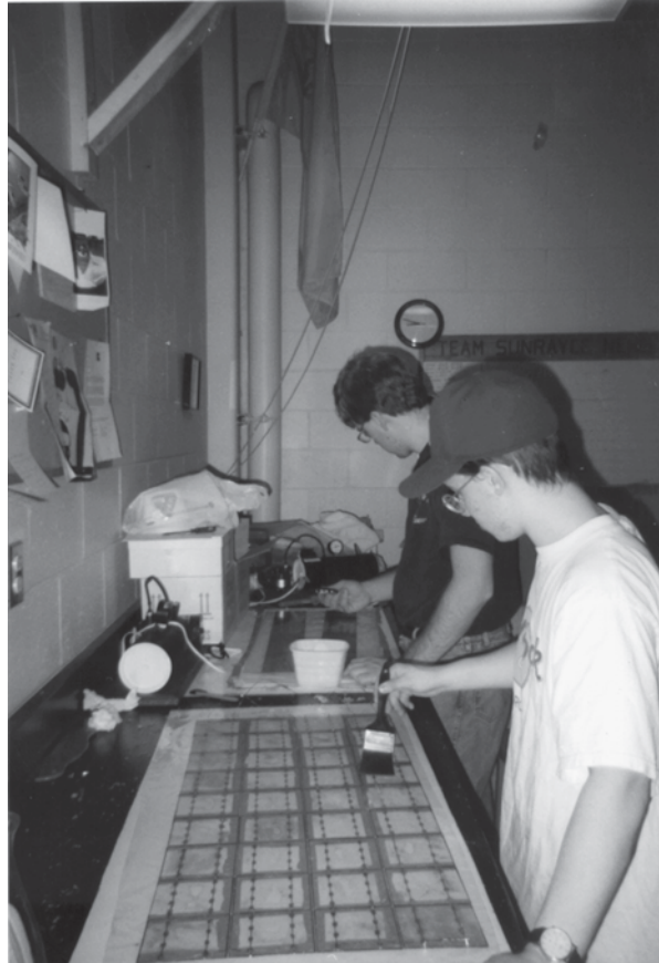
Fig. 11.28 Applying encapsulant. (Brian Lisiescki)
