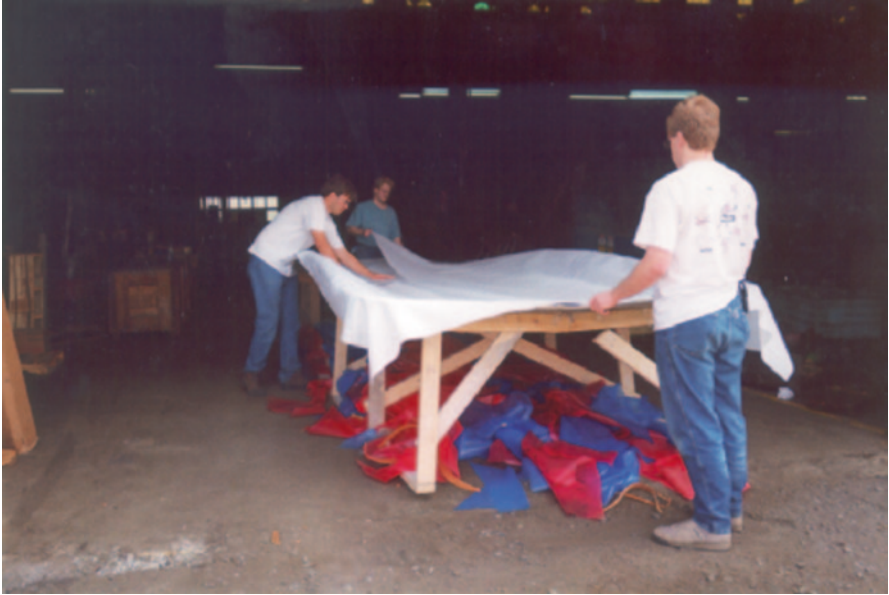
Fig. 11.18 Laying down bleeder cloth. (Brian Lisiecki)
