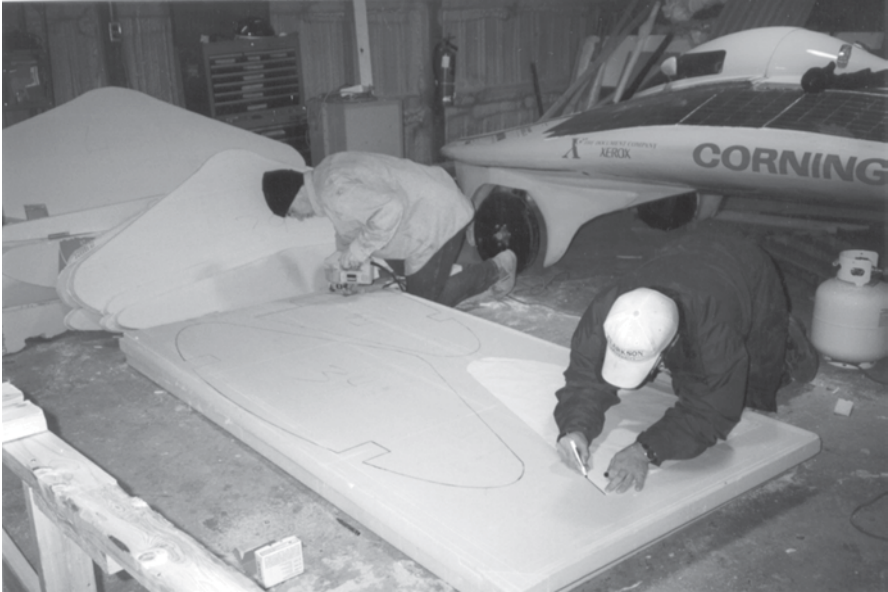
Fig. 11.7 Cutting plug foam segment. (Brian Lisiescki)
