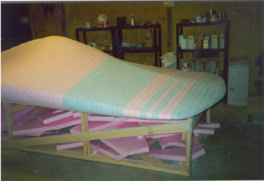
Fig. 11.9 Shaped foam core. (Brian Lisiecki)
