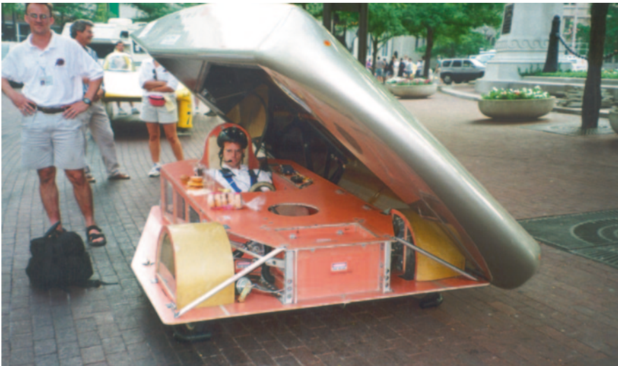
Fig. 11.4 Aluminum honeycomb chassis—Minnesota 1995. (Jules LeDuc)
