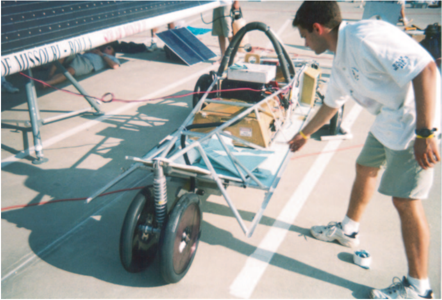
Fig. 11.3 Aluminum space frame—Missouri-Rolla 1999
