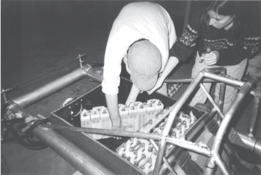
Fig. 11.35 Installing batteries. (Brian Lisiecki)
