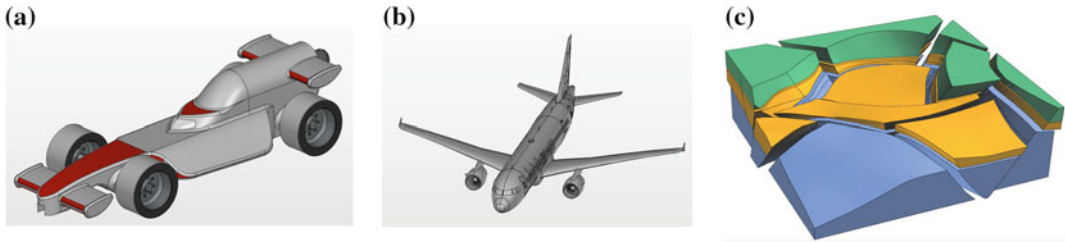
Fig. 4.3 Classical constructive solid geometry and parametric surfaces can be used to model manufactured objects (a) and (b) but are generally not used to represent
