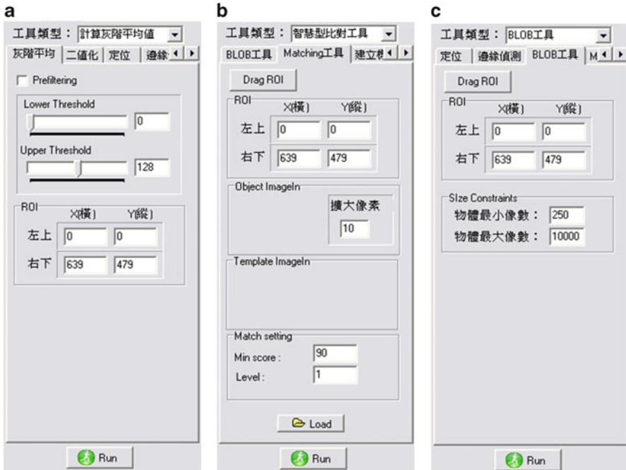
Fig. 52.9 (a) The average gray level tool, (b) the smart matching tool, (c) the BLOB tool and the relevant parameters
