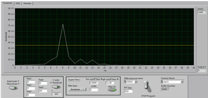
Fig. 61.5 Threshold decision and frequency response of EEG
