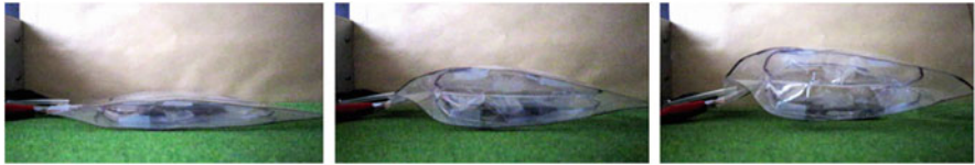
Fig. 9.4 Transient view of movement of the tested actuator when the input voltage of 10 V is applied (Time: 5, 10, 15 s)
