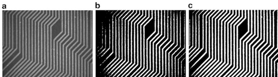
Fig. 52.6 (a) The sample image of TAB surface circuits to be inspected by the thresholding tool. (b) Processed result using a fixed threshold, 128. (c) Processed result using the adaptive threshold
