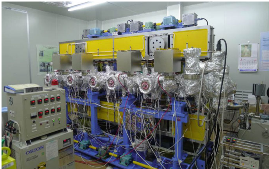
Fig. 18.1 TPS in-vacuum undulator bake-out in the laboratory
