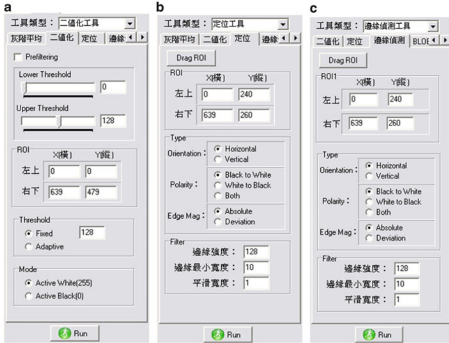
Fig. 52.5 (a) The thresholding tool, (b) the positioning tool, (c) the edge detection tool and the relevant parameters
