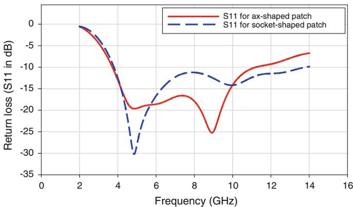
**Fig. 2** Comparison between simulated  $S_{11}$  for ax-shaped and socket-shaped patch antennas
