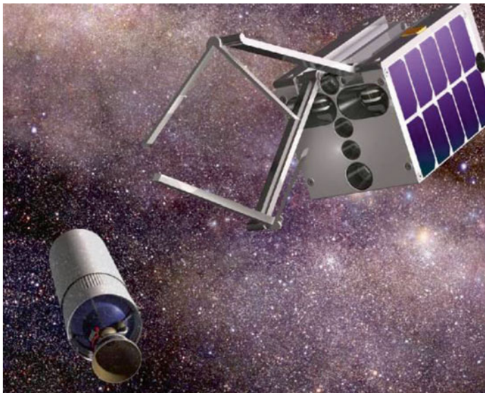
Fig. 5.2 The EDDE Net manager at end of tether system (Graphic courtesy of STAR Inc.)
