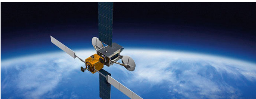
Fig. 2.8 Artist rendition of Vivisat mission extension vehicle mated to a satellite in orbit (Graphic courtesy of Orbital ATK)
