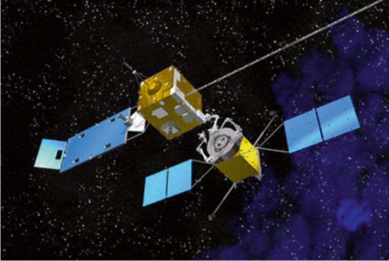
Fig. 2.9 Simulated image of MDA space infrastructure serving vehicle attaching to client satellite (Graphic Courtesy of McDonald Dettwiler Associates)
