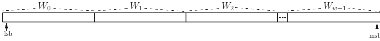
Fig. 1. A wide word in the Ultra-Wide Word architecture. The wide word is divided in w blocks of w bits each, shown here in increasing number of block from left to right.
